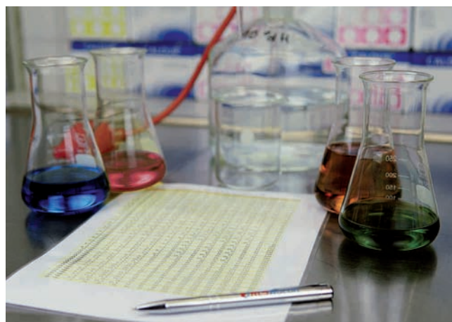
CALDUR®-Test set total hardness GH 100 red-blue Measured value per drop: 1.0 / 0.5 °dH
