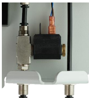
Picture: View of the solenoid valve (no reagent bottle installed)
