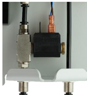
Figure: View of the solenoid valve (no reagent bottle installed)
