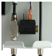
Figure 3: View of the solenoid valve (no reagent bottle installed)
