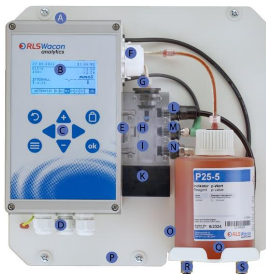
Figure 22: SYCON P analyser with inserted reagent bottle
