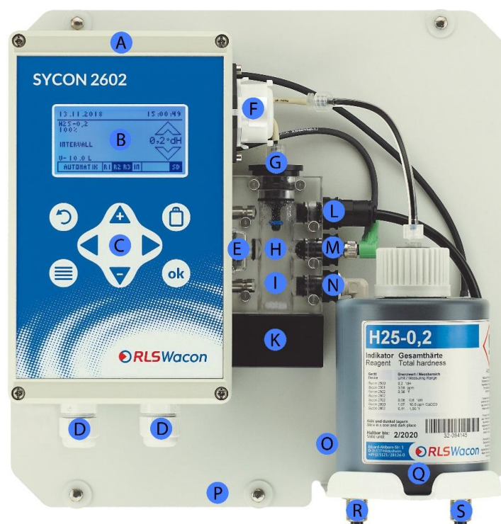
Figure: SYCON 2602 analyzer with installed reagent bottle
